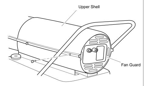
Figure 6 - Upper Shell Removal, 150,000 BTU/Hr Model
